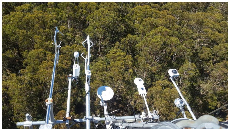
Photos of 70m Tumbarumba Flux tower, and configuration of the albedometers (extreme right). Courtesy of Dr William Woodgate, CSIRO Australia
